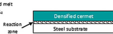
Fig. 13 Proposed mechanism for sinter bonding between 1018 steel and boride based cermets
